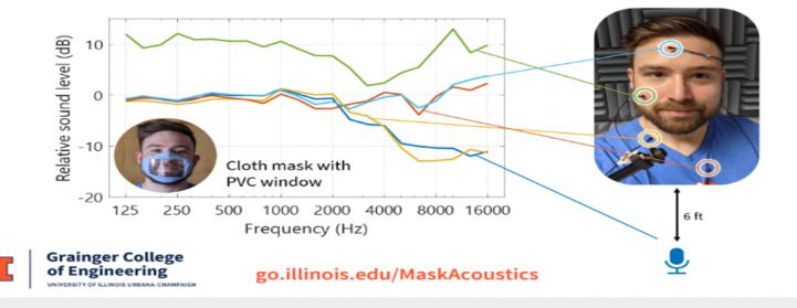
Acoustic effect of the PVC window mask on microphones in different locations on and near the body
